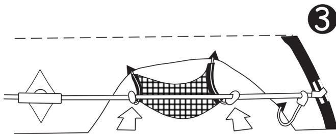
Included with this kite you will also receive two "wind brakes". These are gauze pieces that are attached to both sides of the lower leading edge using the inner and center standoffs, (see diagram 3). By placing these "brakes" on your "Jam" you can SLOW the effects of strong, fast moving winds. This wind "braking" effect, is especially desirable for beginners and novices and will give the flyer additional time to adjust his/her steering lines even in strong winds.
