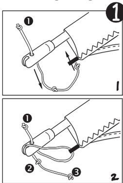
using a tensioning cord. After assembly, the knots and cord ends are tucked away inside recesses specially provided for this purpose, so that you achieve a clean finish. There's also a neat way of attaching a trick cord here.
